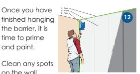
on the wall before priming. Select the primer and paint color. Then, prime and paint your wall covering as you would any other wall, following the directions on your primer and paint.
